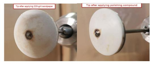
• Cover rehabilitation takes approximately 15 minutes. With clean covers you should be able to run in excess of 2,000in3 of Argyle Materials, well above the 650in3 recommend by SSYS.
