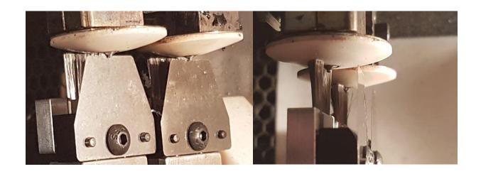
Both flickers and brushes should be replaced when the top edges of them are no longer straight. A small amount of wear on a flicker is acceptable. The flicker should be replaced if it becomes notched or bent. Frayed brushes are acceptable so long as it is even across the top.
